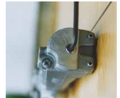
Briton 2003V power adjustment
