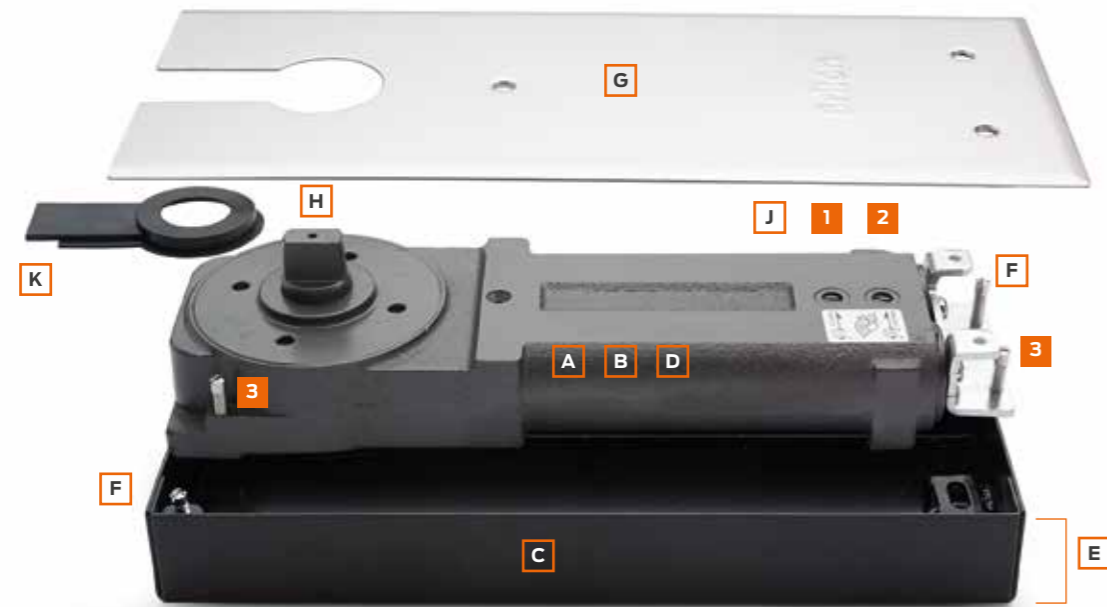
Adjustments: 1 - Closing speed (from 130° opening); 2 - Latch action; 3 - Lateral & vertical adjustment of the closer
