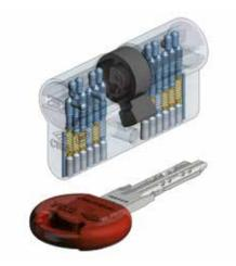
The built in clutch function as standard, allows the cylinder to be operated even if a key is inserted in the opposite side of the cylinder.
