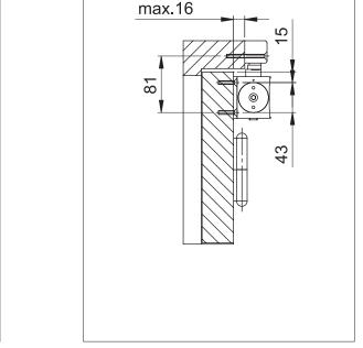
The carry bar is fitted to the passive leaf on the push side of the door. If the passive leaf is opened first it ensures that the active leaf is partially opened to enable the passive leaf to re-close first.
