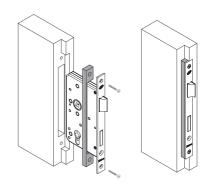
3) Prepare frame to accept Rebate Strike Assembly. Secure assembly with Screws provided.
