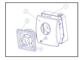
2. Fit the magnet box (1) to the wall or fixed surface. Check that the screw fixings and the mounting surface are strong enough to withstand the holding force of the door retainer.  Cable entry can be directly through the back face of the box or through the 20 mm entries provided for surface mounted pyro or conduit.
