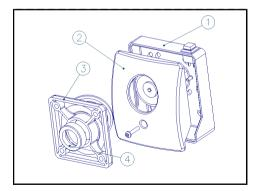
Fit the magnet box (1) to the wall or fixed surface. Check that the screw fixings and the mounting surface are strong enough to withstand the holding force of the door retainer. 3. Cable entry can be directly through the back face of the box or through the 20 mm entries provided for surface mounted pyro or conduit.
