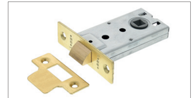
Latch - B3708 & B3709LK ▪ Mortice latches for lever or knob furniture ▪ Meets the requirements of EN 12209 (B3708) ▪ CE marked (B3708) ▪ Accepts bolt through fixings at 38mm centres ▪ 8mm high strength follower
