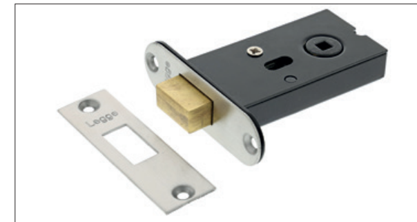
Bathroom Deadbolt - B2515MM/ & B25128MM/ ▪ Mortice bathroom deadbolt with thumbturn operation ▪ Brass deadbolt with thumbturn operation ▪ Accepts bolt through fixings at 38mm centres ▪ Available with 5mm or 8mm follower ▪ Round or square forend and strike
