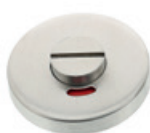
Product Ref: 4210 4211 Function: Bathroom turn & indicator Bathroom extended turn & indicator Description: Ø52 x 8mm with 5mm spindle and bolt through fixings for doors 38 - 44mm
