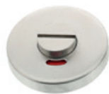
Product Ref: 4210 4211 Function: Bathroom turn & indicator Bathroom extended turn & indicator Description: Ø52 x 8mm with 5mm spindle and bolt through fixings for doors 38 - 44mm
