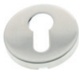
Product Ref: 4213.8.SS 4214.8.SS 4215.8.SS Function: Euro profile cylinder escutcheon Lever key escutcheon Blank escutcheon Description: Ø52 x 8mm with snap on cover. Supplied as pairs as standard. Bolt through fixings supplied as standard suitable for doors 44mm-54mm. Alternative fixings available.
