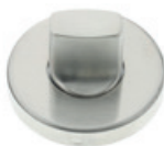
Product Ref: 4210 4211 Function: Bathroom turn & indicator Bathroom extended turn & indicator Description: Ø52 x 8mm with 5mm spindle and bolt through fixings for doors 38 - 44mm
