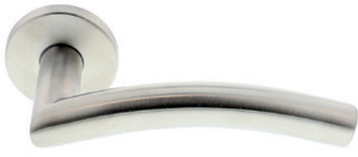
4205.19.SS Curved mitred Ø19mm round bar lever handle on rose with bolt through fixings at 38mm centres.
