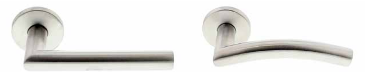
4204.19.SS Straight mitred, Ø19mm round bar lever handle on rose with bolt through fixings at 38mm centres. 4205.19.SS Curved mitred Ø19mm round bar lever handle on rose with bolt through fixings at 38mm centres.
